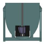
'U' Shaped Tank avoids sanding at the corners, maximizes utilization of the tank volume. It avoids dead zone & helps in smooth restart of the equipment after any sudden stoppage.
