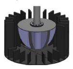
The MBE Flotation cell's mechanism disperses the air in the slurry and also keeps the slurry in a complete suspension by its pumping action. The mechanism consists of a rotor coupled to a hollow shaft and a stator attached to the base of the tank. The shaft is connected to a bearing unit, which is driven by an electric motor & power transmission through a V-belt drive. Air is fed through the hollow shaft and exits through outlets in the rotor.
